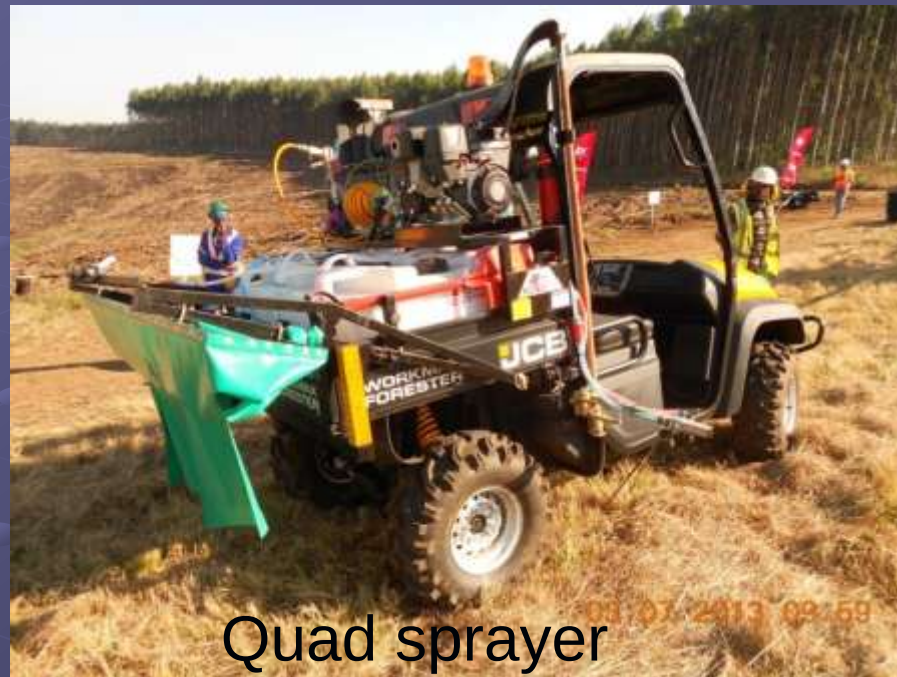
Self levelling boom sprayer
